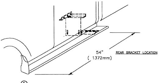
MEASURE FROM FRONT WHEEL WELL TO BRACKET LOCATION MARK THIS DIMENSION ON THE PINCH WELD
