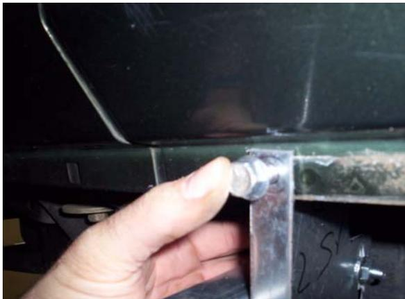
Insert a 5/16" flange bolt trough pinch weld and FL223 and FL232 tighten with a 5/16" flanged nut.
