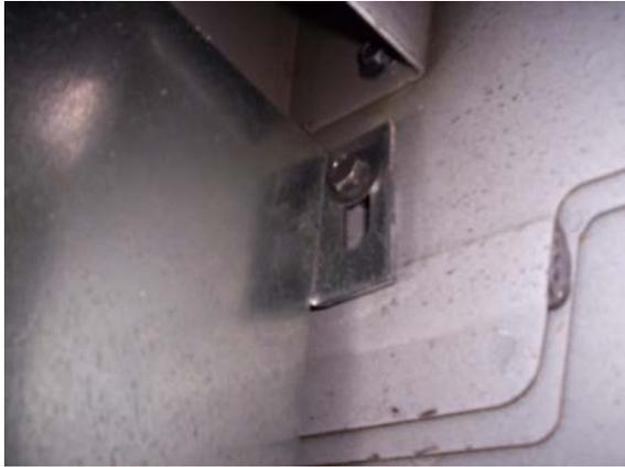
At 102" location on pass side remove factory 10mm bolt and reinstall through slot in FL232
