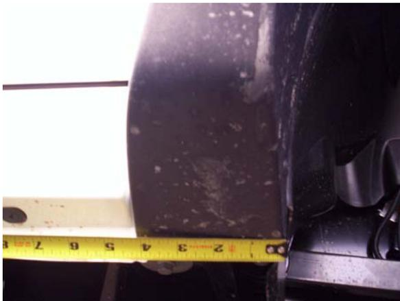
Measure from front wheel well back making a mark on the pinch weld at (**Pass side 10", 22", 38", 50", 70", 88" 100"**) (**DR side 7", 19", 36", 49"**)
