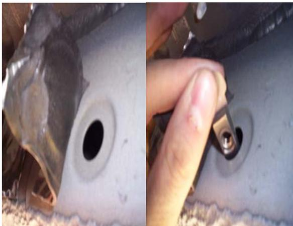
Remove tape from underbody to install 8mm pull nut at 22" 38" DR side, and 7" 19" 36" 49" pass side.
