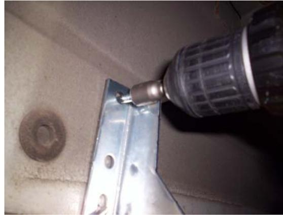
At remaining locations install two self tapping bolts through slot in FL223
