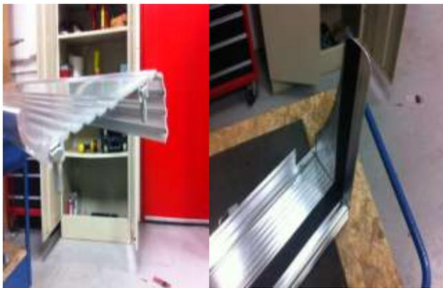
**STEP 8:** Starting on the very top edge of the running board apply included trim lock the entire length of the board. Slide the open end of the seal over the board and press firmly every few inches
