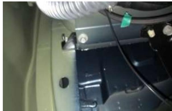
**STEP 5:** Replace bolt through front hole in the bracket and install a self tapping 3/8 screw through cross member for rear hole. Make sure foot of bracket is pointing outward. Attach 3124F the same as the previous brackets.
