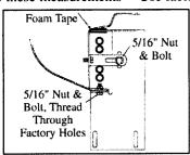
5. Place foam tape at top of FL29 flat plate. Bolt to AS02 then to pinch weld with 5/16" nuts and bolts. Note: top of flat plate must hit rocker panel. Tighten FL29 to AS02 and 8mm bolt before tightening to pinch weld. Note: On 2005 models, front and rear brackets attach using the factory stud and nut supplied in bolt kit.
