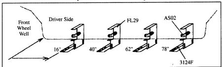
3. Measure from front wheel well, back 16", 40", 62" and 78". Mark these bracket locations. Note: Steel plates have been inserted under fiberglass to mount brackets securely using self-drilling screws. Note: Factory holes should be close to these measurements -- Use factory holes only.
