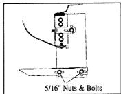
6. Attach 3124F step support to flat plate using two 5/16" nuts and bolts. Do not tighten at this time.
