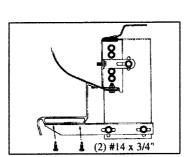
9. Use #14 x 3/4" self-drilling screws to fasten GlaStep to step supports, then tighten all bolts to 18 foot pounds
