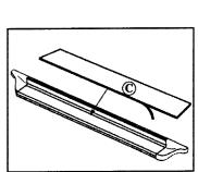
10. Tighten step support bolt and nut to 18 foot pounds. Place pad on step. Peel off tape backing to secure. Don't forget the Owens label!
