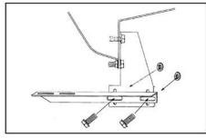
Attach 3124F step supports to FL11 using 5/16" washer head bolts and nuts.
