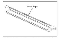
**6.** Apply foam tape strips to top GlaStep edge.
