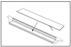
Place step pad on GlaStep. Peel off tape backing to secure. Don't forget the Owens label!
