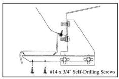
Secure bracket to GlaStep with two #14 x 3/4" self-drilling screws per bracket.
