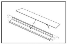
Place step pad on GlaStep. Peel off tape backing to secure. Don't forget the Owens label! IN121A 5/1/07
