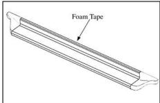
Apply foam tape strips to top GlaStep edge.
