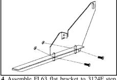
Assemble FL63 flat bracket to 3124F step support using two 5/16" nuts and bolts. Do not tighten at this time.
