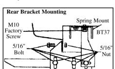
**6.** Remove the front inside spring mount M10 bolt, reinstall mounting the BT37 bent tab. Use a 5/16" bolt and nut to attach to flat bracket FL71. Drill a 5/16" hole through the bracket and into the pinch weld. Secure with a 5/16" bolt and nut.
