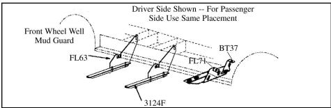
Steel plates have been inserted under fiberglass to mount brackets securely using self-drilling screws. See illustration at right. Follow instruction steps #5 and #6 for bracket locations.
