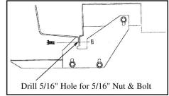
7. Pull flat brackets up tight to body. Drill 5/16" diameter hole using bracket hole as a guide, then through pinch weld. Secure with 5/16" nut and bolt.
