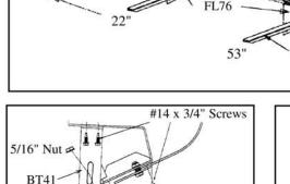
5A. Attach BT41s to FL76s using 5/16" nuts and bolts. Mate top of BT41s to bottom of step areas. Screw BT41 to bottom of step area using two #14 screws, then screw through FL76 into pinch weld using one #14 screw. Snug 5/16" nut and bolt.
