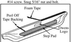
Clean surface prior to attaching tape and step pads with denatured alcohol. Apply foam tape to top lip of board. Position step pad on stepping surface. Peel off tape backing starting with rear strip. Keep pad in position, peel off backing then apply pressure to top of pad to stick tape to board. Continue above steps for all tape strips.
