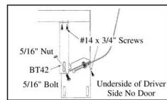
5B. When no rear drivers door is present, use BT42s in place of BT41s.
