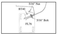
4. Mate BT40 top clamp onto FL76 flat plate using 5/16" nuts and bolts. Clamp assembly onto pinch weld at marks.
