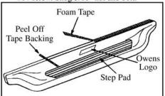
Position step on brackets. Align back of step upper lip approximately 1-1/2" out from edge of pinch weld. Use #12 x 3/4" screw through lip. (Note: If installing box boards, align both before securing steps to body.) Next, attach step to 3124F using two #14 x 3/4" screws. Adjust brackets and tighten all bolts to 18 foot pounds.
