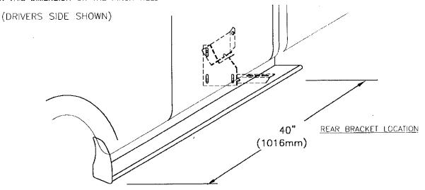
BRACKET ASSEMBLY ASSEMBLE WITH 5/16" BOLTS LEAVE BOLTS LOOSE
