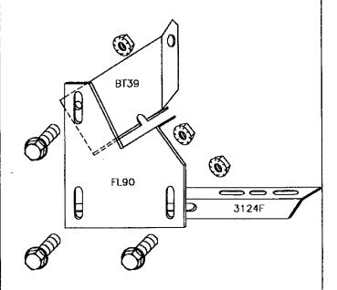
BRACKET ASSEMBLY MOUNT TO BODY ASSEMBLE WITH 5/16" BOLTS AND #14 SELF DRILLING TEK SCREWS
