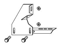
BOX BRACKET ASSEMBLY, 8' BOX ONLY ASSEMBLE WITH 5/16" BOLTS
