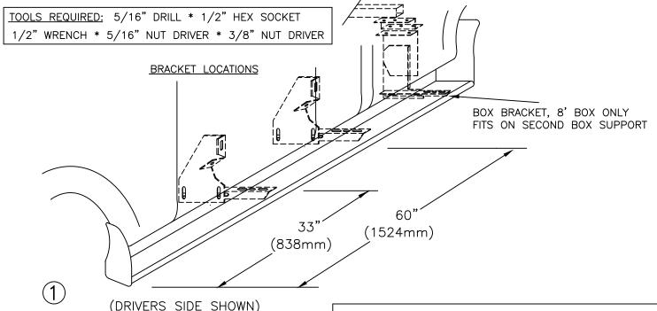
MEASURE FROM FRONT WHEEL WELL TO BRACKET LOCATIONS. MARK THIS DIMENSION ON THE PINCH WELD
