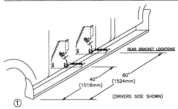
MEASURE FROM FRONT WHEEL WELL TO BRACKET LOATIONS. MARK THIS DIMENSION ON THE PINCH WELD
