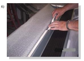
Attach foam tape to the top lip of the board where it meets up with the body. Attach step tread and logo also.
