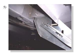
Attach one channel bracket with 5/16 bolts and nuts on each flat bracket. Snug but do not tighten.
