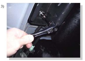
Remove the two forward bolts of the rear control arm holder. Do not discard, these will be used to attach rear bracket.
