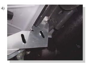
Attach FL127D using bolts removed in step3. From back side of pinch weld drill 5/16" hole through pinch weld to line up with the hole in the bracket . Insert a 5/16" bolt and fasten with nut . Tighten all bolts.
