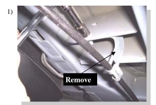
On the driver side at 25" (23" on passenger side) back from wheel well, remove factory bracket holding the emergency brake cable.
