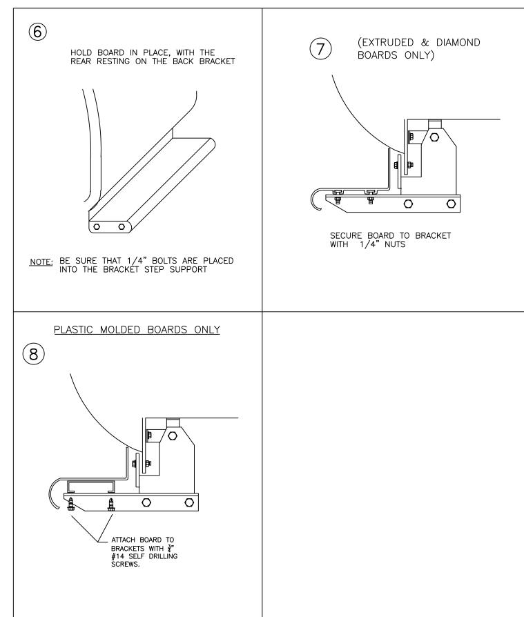
WITH BOARD LEVEL TIGHTEN ALL LOOSE BOLTS
