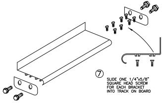
BOARDS WITH WELDED END CAPS WILL ONLY NEED TO SLIDE IN THE BOLTS INTO THE TRACK IN THIS STEP.
