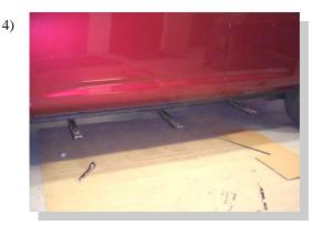
Attach brackets in their proper location. Attach the front bracket with the bolt removed in step one, for the middle and rear bracket attach with one 8mm bolt. Do not tighten yet.
