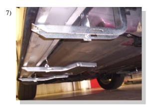
Place the board on the brackets and align from front to back and level the board. Tighten <u>all</u> loose bracket bolts now.
