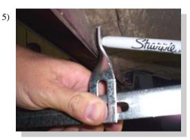
Holding a twisted strap to each bracket and pinch weld, make a mark on the pinch weld. At each mark drill a 23/64" hole through the pinch weld.
