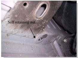
Install one self retaining nut towards the rear of the vehicle in the hole shown just in front of the rear suspension.
