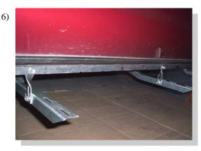
Attach twisted strap to the bracket and vehicle with 5/16" flanged bolts and nuts. The twisted strap can go on the front or back side of the pinch weld. Do not tighten yet.
