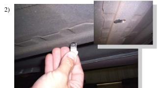
Measuring from the same spot as in step one, at approximately 28" install one self retaining nut as shown in factory hole.
