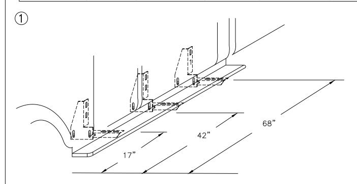
(DRIVERS SIDE SHOWN) MEASURE FROM FRONT WHEEL WELL TO DIMENSIONS SHOWN THERE ARE FACTORY HOLES AT OR VERY CLOSE TO THESE LOCATIONS
