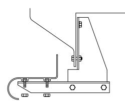
SECURE BOARD TO BRACKET WITH 1/4" NUTS
