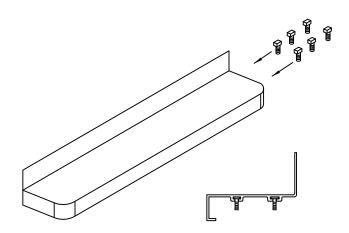
SLIDE ONE 1/4" X 5/8" SQUARE HEAD SCREWS INTO EACH TRACK FOR EACH BRACKET.
