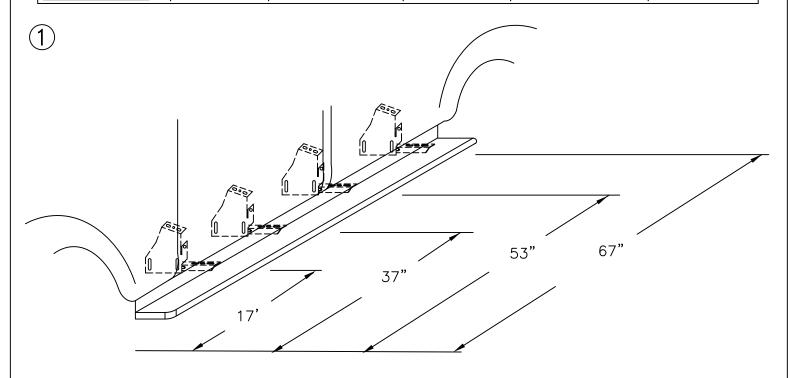
(DRIVERS SIDE SHOWN) MEASURE FROM FRONT WHEEL WELL TO DIMENSIONS SHOWN
