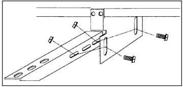
**3.** Assemble bracket components with 5/16" nuts and bolts as shown. **Do not tighten at this time.**
