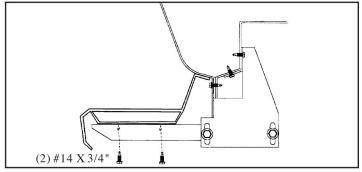
5. Secure step support bracket to bottom of board using two #14 x 3/4" self-drilling screws per bracket. **Tighten all bolts to 18 foot pounds.**
