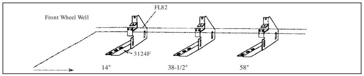
1. Measure from front wheel well, back to dimensions shown above. Mark these bracket location centers.
