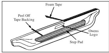
**4.** Clean surface prior to attaching tape and step pads with denatured alcohol. Apply foam tape to top lip of board. Position step pad on stepping surface. Peel off tape backing starting with rear strip. Keep pad in position, peel off backing then apply pressure to top of pad to stick tape to board. Continue above steps for all tape strips.
