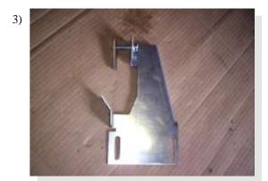
Assemble brackets as shown using one long 5/16" bolt and steel retaining nut. (FL149 shown)
