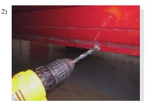
At each of the locations from step one, drill a 5/16" hole through the pinch weld.
