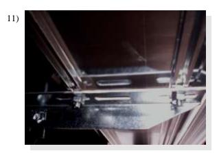
Place the board on the brackets with bolts through slots. Attach with 1/4" nuts.
