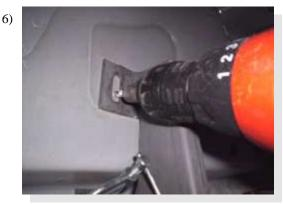
For the Standard Cab bracket (FL146) at the 48" location, it will be necessary to attach the bracket with a self drilling screw
