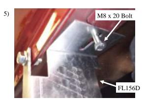
Attach bracket with 1 slot to vehicle at measured location 62". The rear locations use an 8mm bolt and a factory threaded hole. Straighten bracket and bolt through pinch weld.
