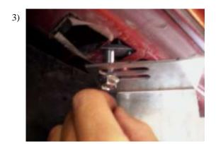
You will need to insert the re-enforcement nuts into hole under vehicle at the measured locations as stated in Fig. 1
