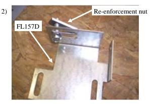
Attach bolt and re-enforcement nut onto the bolt engaging a couple threads as shown. Brackets with 2 slots are for the <u>front</u> and <u>middle</u> locations and the bracket with 1 slot is for the rear location.
