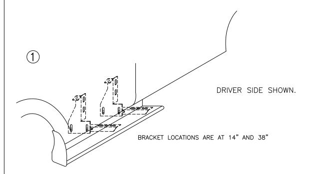
MEASURE FROM FRONT WHEEL WELL TO BRACKET LOATIONS. MARK THIS DIMENSION ON THE PINCH WELD
