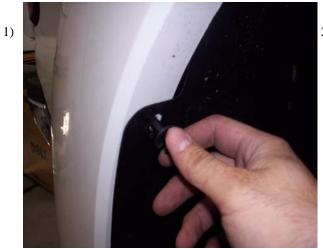
Start by removing push pin in rear inner plastic wheel well cover.
