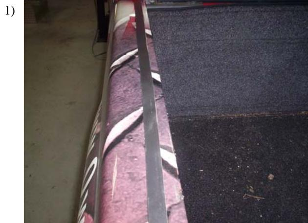
Start by placing the foam tape, on the bed rails where you are placing your tool box.
