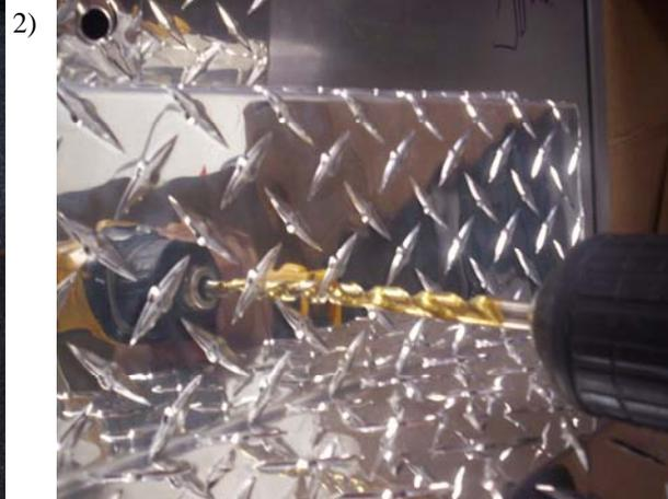
Center tool box and make a mark on bottom of tool box 1/4" from bed rail (on both sides). Remove box and drill a 5/16" hole.
