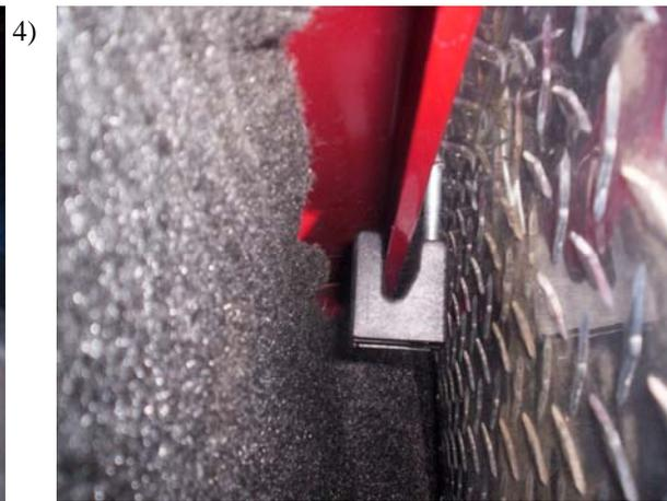
Attach plastic U-clamp to 5/16" bolt and tighten.
