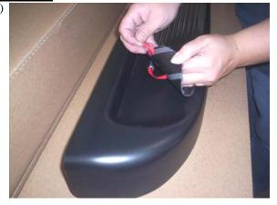
Position step tread where you want it. Then holding step tread in place remove adhesive cover one row at a time and press firmly to hold in place.
