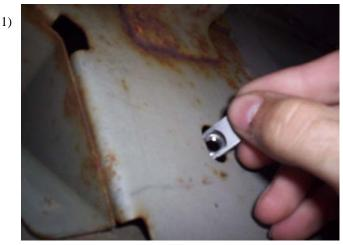
Measure back from the front wheel well on driver side 69" and make a mark on the pinch weld, drill a 5/16" hole.
