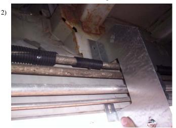
Attach the FL199 for 2" riser boards or the FL201 for the 4" riser boards by inserting either an 8mm bolt through the top hole in the bracket into the pull nut, or, if there is no hole for the pull nut, use the self drilling screw. Insert 5/16" flanged bolt through the hole in pinch weld and through slot in FL199 and tighten. Follow the rest of the steps in the other instruction sheet for board installation.
