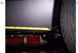
Measure from front wheel well towards the rear and make a mark on pinch weld at 14" 31" 44" 59". At these locations you will have to notch the plastic body molding so you can drill a 5/16' hole through pinch weld.
