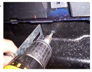
After you installed all the factory 10mm bolts back in place, install a self tapping screw on each side of the bracket where you made a slit in the splash shield.
