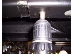
Remove plastic splash shield on the under body, by removing all the 10mm bolts holding in place. There is one on both sides of vehicle. Save bolts and splash shields for reinstall.
