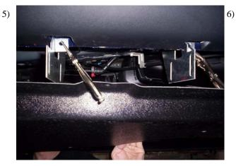
After all FL202's are installed you will have to cut a slit in the splash shield at the 44" bracket location, so you can reinstall the splash shield around the bracket.
