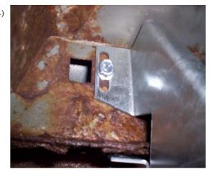
Insert a 5/16" flanged bolt through bracket and attach to clip nut. Some vehicles you will not have this hole, so you will have to use a self tapping bolt.
