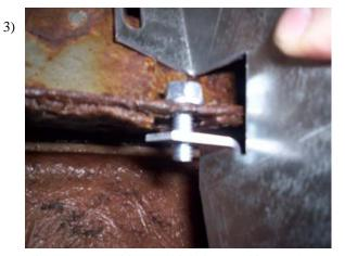
Install BRKT assembly to vehicle by attaching FL47 at 13" measurement and FL46D/P (D-Driver side, P-Passenger side) at the remaining measurements. Insert 5/16" flanged bolt through factory hole in pinch weld and through brackets and tighten with 5/16" flanged nut. If there is no hole drill a 5/16" hole through pinch weld.
