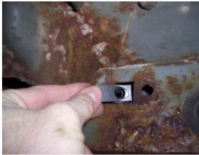
Insert clip nut into body holes at all bracket locations.
