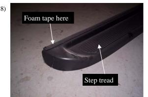
On ABS boards only, apply foam tape and step tread as shown in picture. Center step tread between the ends of the board and keep close to outside edge.
