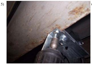
Insert a self tapping bolt through the hole in FL90 into vehicles pinch weld and BT39, and tighten.
