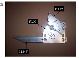
Assemble FL90, BT39, and 3124F with a 5/16 flanged nut and bolt as shown. Snug, but don't tighten yet.
