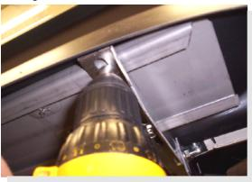
For Molded Boards: Position board where you want it. Install self tapping bolts through bracket into the shoulder of the steel channel on the bottom of the board.
