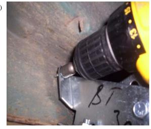
Insert a self tapping bolt through BT39 into vehicle body and tighten. Next tighten the two 5/16" nut and bolts that attach the BT39 and FL90 together.
