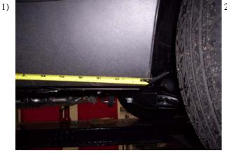
Measure from front wheel well back making a mark on the pinch weld at 17", 38" for STD cab and 17" 40" 62" for EXT cab and 17" 40" 62" 78" for CREW cab.
