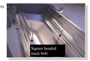
For Aluminum Boards: Insert one square headed track bolt into both tracks for each bracket.
