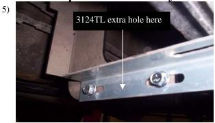
Std cab: Attach 3124TR at Dr rear and pass front location, (NOTE, 3124TL will have extra hole where indicated above.) attach 3124TL at Dr front and pass rear location using 5/16" flanged nut and bolts as shown.
