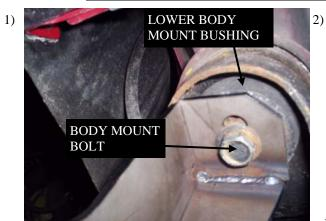
Starting at DR side front body mount. Remove body mount bolt, place FL215 between the bolt and the lower body mount bushing, retighten body mount bolt. Repeat steps for pass side using FL207
