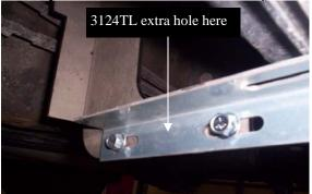
Ext/Crew cab: Attach 3124TR at Dr rear/middle, pass front/middle location, ( **NOTE, 3124TL will have extra hole where indicated above.**) attach 3124TL at Dr front and pass rear location using 5/16" flanged nut and bolts as shown.
