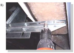
Using self drilling screws attach the board to the angle brackets. Level board and tighten any remaining loose bolts at this time.
