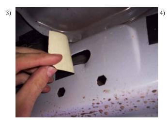
Remove tape from underbody to install reinforcement nut at locations you measured in step 1
