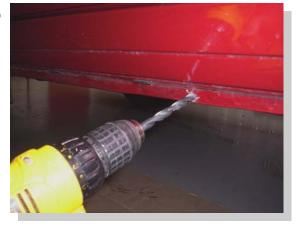
Drill a 5/16" hole in pinch weld at pre-marked location, to insert a 5/16" flanged bolt through pinch weld and FL21.
