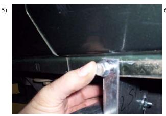
Insert a 5/16" flange bolt trough pinch weld and FL217 and tighten with a 5/16" flanged nut. (BRKT show on outside of pinch weld for picture purpose only)
