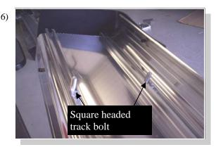
Insert one square headed track bolt into both tracks for each bracket.
