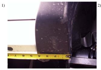
Measure from front wheel well back making a mark on the pinch weld at (STD cab 11" 25" 55" pass side and 11" 55" DR side) (Crew cab 11" 36" 56" 84" pass side and 11"36"84" DR side.)
