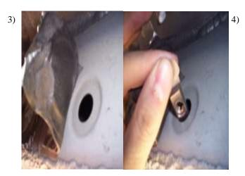
Remove tape from underbody to install 8mm pull nut at 4 1/2" 35 7/8" Driver side, and 4" 20" 35 1/2" Passenger side.
