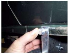
Insert a 5/16" flange bolt trough pinch weld and FL223 and FL232 tighten with a 5/16" flanged nut. (BRKT show on outside of pinch weld for picture purpose only, BRKT mounts to inside of pinch weld)
