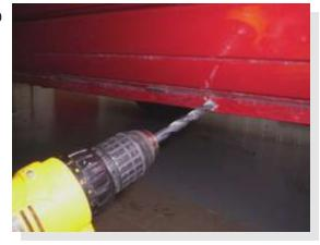
Drill a 5/16" hole in pinch weld at pre-marked location, to insert a 5/16" flanged bolt through pinch weld and FL223 and FL232 (99" on Driver and 98" on Passenger side).
