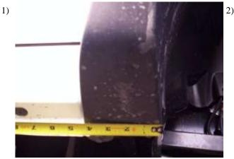
Measure from front wheel well back making a mark on the pinch weld at (DR side 4 1/2", 20 1/4", 35 7/8", 50", 70", 88" 99") (pass side 4", 20", 35 1/2", 45", 70", 85" 99")
