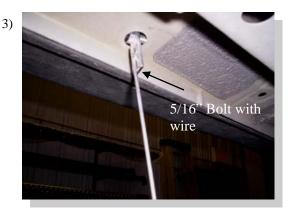
Remove the reward rubber plug and insert the bolt with a wire through the hole as shown. "Fish" the wire towards the rear of the vehicle and insert the bolt through the rear hole.
