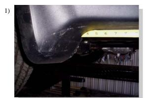
Brackets will be attached using factory mounting locations at 17 1/2", 36" and 58".
