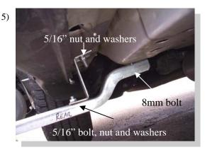
Attach CB64 and "Z" bracket to vehicle as shown at the rear location.
