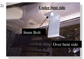
Attach the front two "Z" brackets to factory holes with 8mm bolts. The rear "Z" bracket will attach with supplied bolt/wire and nut. The under bent side of the Z bracket goes against body.
