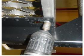
Set board on top of brkts. Center board left to right and insert a self tapping bolt through each of the slots in the brkts into the board.
