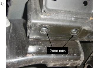
At rear of vehicle find the two 12mm nuts inside the frame rails on each side of vehicle.
