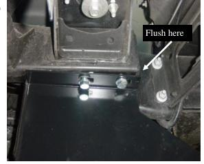
Insert two 12mm bolts with 12mm washer through slot on FL239D/P and into the 12mm nuts in frame rail as shown. Flush FL239D/P flange with back of frame rail and tighten bolts
