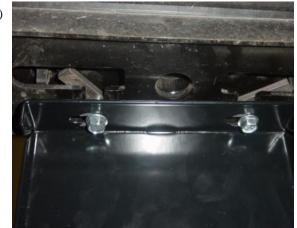
Insert 5/16" flanged bolts through slots with reinforcement nuts. Insert into slots in bumper as shown. With a screwdriver turn the nut on pass side so it is pointing same direction as driver side. Tighten 5/16" flanged bolts.
