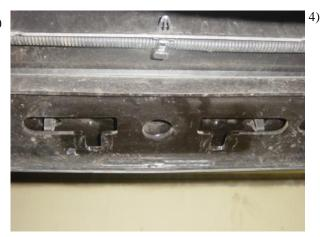
Locate these slots located in the center on the bottom of the rear bumper.
