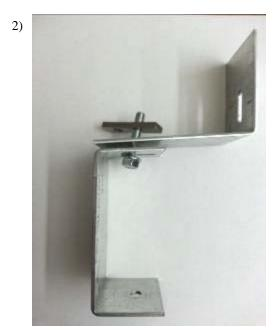
Assemble FL243 and FL244 together as shown using the 1.5" long 5/16" bolt and steel retaining nut. Use the center hole on the retaining nut.
