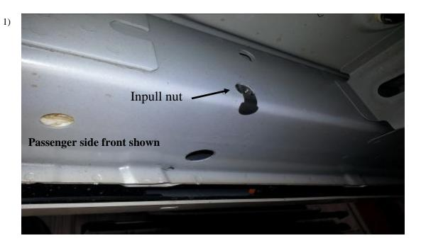
On the underside of the body locate the factory holes as shown. There is a set of these holes at each corner of the underbody. (There may be foam filling in the holes that will need to be pushed into the holes for the fasteners) Insert inpull nut into hole as shown,
