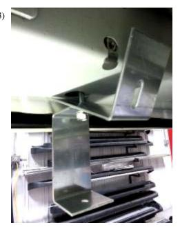
Insert the retaining nut into the factory hole. Leave loose. This will get tightened in the next step.
