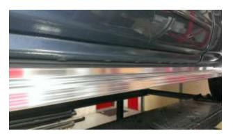
**STEP 10:** Starting with the first bracket location adjust 3124F either up or down to make sure the top of the running board sits flush with the bottom of the vehicle. After the board is level and even front to back, using 3/4" self tapping screws in 3 places each, attach the front and rear mud flap to the inner fender well. Be sure to drill into metal.
