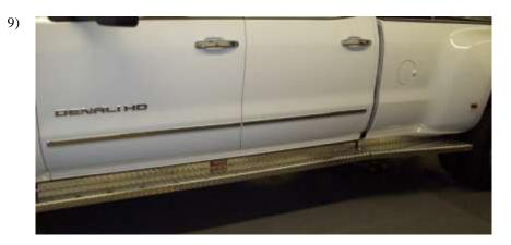
Level boards and tighten all bolts on brackets.
