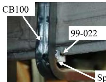
Slide a washer on a 5/16" x 1-1/2" bolt. Then slide the bolt through slot in rear of CB100 and spacer tube between the CB100 and 99-022 then thread into the rear of the pinch weld clamp and tighten up the bolt into the clamp but leave loose for now for adjustment later.
