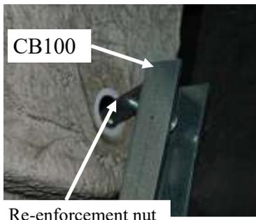
Slide a washer on a 5/16" x 1-1/2" bolt. Then slide the bolt through the top tab of a CB100 and thread a re-enforcement nut only engaging a couple threads and slide nut into hole on rear rocker.
