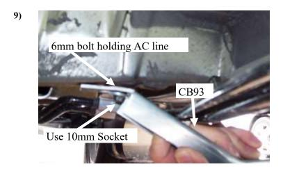
As you look under the vehicle from the front wheel rearward at 20 3/4" locate the bolt securing air conditioning line bracket, remove the bolt with 10mm socket place a CB93 bracket up to hole place the bolt removed through a washer supplied then bolt through slot in CB93 hand tighten bolt. Using a 5/16" x 3/4" bolt through BT67 then through slot in CB93 and secure with nut. Tighten up the bolt into the nut but leave loose for now for adjustment later
