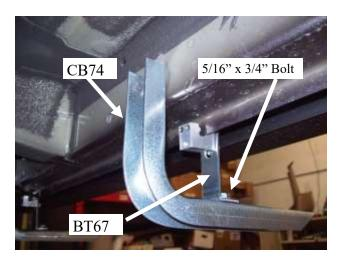
At 36 1/4" remove the rubber plug in the rear of the rocker panel. Insert 5/16" X 1-1/2" bolt through washer then put bolt through CB74 bracket and thread into short reenforcement nut. Slide nut into hole in rear of rocker panel as shown hand tighten bracket up to rear of rocker. Using a 5/16" x 3/4" bolt through BT67 then through slot in CB74 and secure with nut. Tighten up the bolt into the nut but leave loose for now for adjust-
