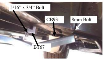
As you look under the vehicle from the front wheel rearward at 20 3/4" locate the two bolts securing the fuel tank barrier bar, remove both bolts with 13mm socket place a CB93 bracket up to hole toward the out side of vehicle place the bolt removed through slot in CB93 hand tighten bolt. Using a 5/16" x 3/4" bolt through BT67 then through slot in CB93 and secure with nut. Tighten up the bolt into the nut but leave loose for now for adjustment later
