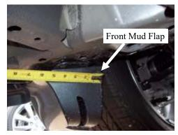
Measure from the Front wheel well back and make a mark on the pinch weld at 20 3/4", 36 1/4", and 60.0" on both sides. At each mark mount the pinch weld clamp, by tightening the set screws with 1/8" Allen wrench holding with pair of vise grips for leverage.
