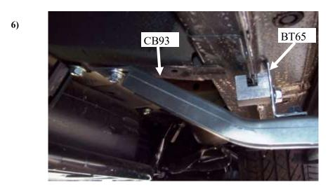
Attach a CB93 to the BT65 one 5/16" x 3/4" bolt and nut to the angle bracket. Hand tighten all bolts.
