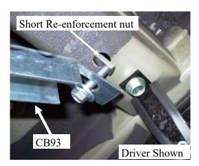
At 60" from front, insert 5/16" X 1-1/2" bolt through washer then put bolt through top tab of the CB93 bracket and thread into short re-enforcement nut. Slide nut into hole in frame then hand tighten as shown for 3rd bracket position.
