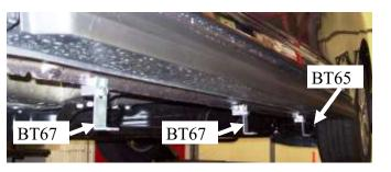
At each pinch weld clamp attach one BT67 angle bracket on front and center and BT65 in rear as shown with a  $5/16 \times 3/4$ " bolt.
