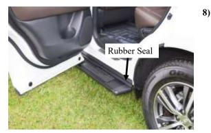
Position board between wheel wells front will touch back of the front mud flap.
