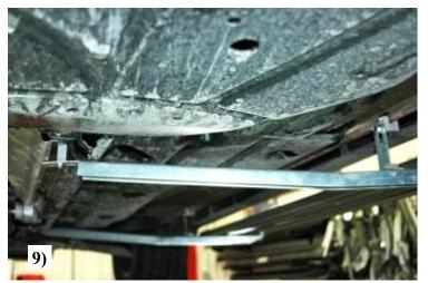
9) With the board on the brackets and align from front to back and level the board. Tighten <u>all</u> loose bracket bolts now.
