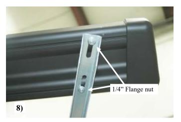
8) Slide the end cap off the board then slide (1) hex head bolt into both the front track and rear track for each bracket location. Replace end cap and screw as shown in board instructions. Put 1/4" flange nuts onto bolts and center the board on the vehicle and tighten nuts to secure board to the brackets.
