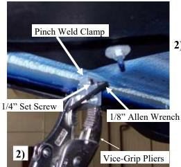
2) At each mark mount the pinch weld clamp, you will have to pry the lower plastic away from pinch weld metal to fit clamp onto pinch weld metal, then by tightening the set screws with 1/8" Allen wrench holding with pair of vise grips for leverage.
