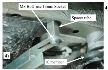
4) For 1st position on both side locate the bolt between K member and exhaust hanger, loosen and remove the bolt with 13mm socket.
