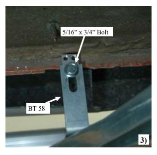
Mount BT 58 to pinch weld clamp with 5/16" x 3/4" bolt
