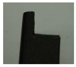
5A) For a Ford Super Duty truck notch top 1" x 1" cutting with diagonal cutter nipping about 1/4" at a time, or cut with saw if available.
