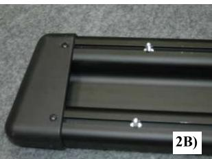
2) After all bolts are in track for all the bracket locations, slide the end cap onto Fusion board with the wider of taper toward the rear of the board. Picture 2A Once end caps are on all the way and square take a Phillips bit in drill and secure with self tapping screws into track area repeat for the other end. Picture 2B
