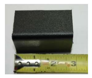
**5B)** For a GM truck cut down to 2 3/4" with diagonal cutter nipping about 1/4" at a time, or cut with saw if available.
