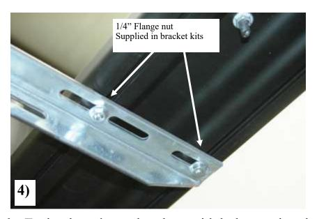
4) Place the Fusion board onto brackets with bolts coming through slots in brackets and put nuts onto bolts. Slide the board so that it is centered and level on the vehicle then tighten all nuts.
