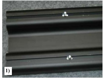
1) Slide hex head bolt into both the front track and rear track for each bracket location.
