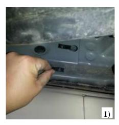
1) At each of the measurements above remove the rubber plug in the holes and slide 5/16" spring clips supplied in bolt package into the larger hole slide toward the smaller hole until clip snaps into position.
