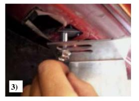
Insert the re-enforcement nuts into hole under vehicle at the measured locations as stated in **Picture #1**
