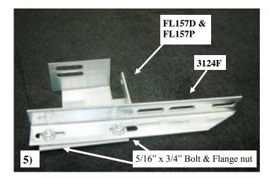
Attach a 3124F angle bracket to the FL157D and FL157P with 5/16" bolts and nuts. Snug but do not tighten at this time. **Picture #5**
