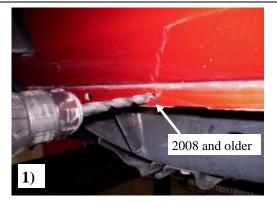
The bracket locations should be measured from front of <u>pinch weld</u> to approx. locations. The front 12", middle 36 at rear .You may need to drill for clearance. **Picture #1**
