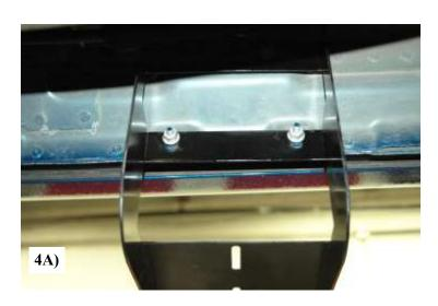
Slide plastic washer onto each of the 3 studs then slide the FL273 bracket over the studs on the back of the rocker panel. **Picture 4A**Place three M8 Flange nuts supplied in bolt package onto the studs. **Picture 4B**
