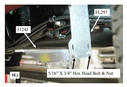
Place the 3124J angle bracket onto the FL297 bracket and secure to each other with two 5/16" x 3/4" hex head bolts and two flange nuts. **Picture 5E**
