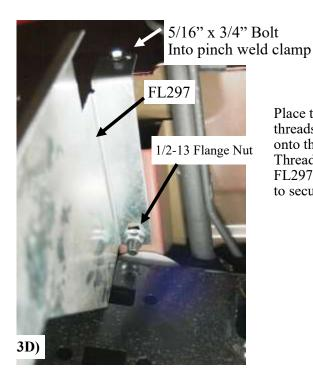
Place the FL297 bracket up so the rear slot fits onto the threads of the 30-3410 then thread the 1/2-13 flange nut onto the threads of the 30-3410 stud plate. **Picture 3D** Thread a 5/16 x 3/4 flange bolt through the top slot of the FL297 and into the pinch weld clamp 99-022 tighten both to secure bracket to the vehicle. **Picture 3D**
