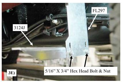
Place the 3124J angle bracket onto the FL297 bracket and secure to each other with two 5/16" x 3/4" hex head bolts and two flange nuts. **Picture 3E**
