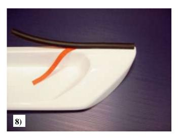
8) Apply foam tape to top edge of board
