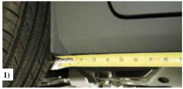
1) Measuring from the back side of the front mud flap as shown in photo. Mark the inside of pinch weld with marker.
