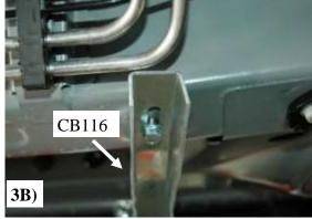
Mount a CB116 using a 5/16"x1-1/2" bolt through CB116 thread into short re-enforcement nut then slide nut into the hole in the frame. Hole at 11 1/2" from front wheel well. (Photo 3A)
