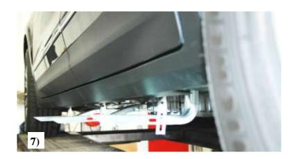
7) Place the board on the brackets and align from front to back and level the board.
