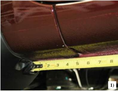
1) Measure back from front wheel well as seen in **Picture 1**, at the distance of 13-1/2", 29-1/4", 45" and 68" you will see M6 bolts at 13-1/2", 29-1/4", 45" locations on the underside of body just behind the pinch weld, and a round hole at 68" location on inside rocker panel. This is where the brackets top tab will be placed.
