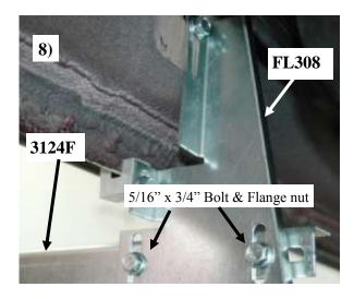
8) Attach a 3124F angle bracket to the FL308 with 5/16" bolts and nuts. Snug but do not tighten at this time. Picture #8
