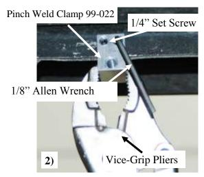
2) At each center mark, mount the pinch weld clamp 99-022. Tighten the set screws with 1/8" Allen wrench holding with pair of vise grips for leverage.
