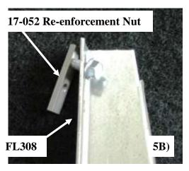
**5B)** Place a 5/16" x 3/4" flange bolt through the top slots on the FL308 bracket and thread a couple threads into 17-052 re-enforcement nut. **Picture 5B**
