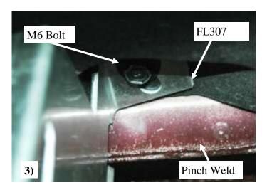
3) Remove the M6 bolt on the underside of vehicle For the first three positions with 10mm socket. Place the FL307 bracket up to hole where bolt was removed and replace the M6 bolt through the top tab of the FL307 bracket.
