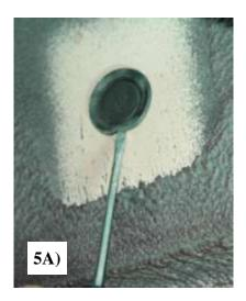
**5A)** Remove the rubber plug in the rear of rocker panel at 68" with a screw driver.
