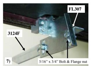
7) Attach a 3124F angle bracket to the FL307 with 5/16" bolts and nuts. Snug but do not tighten at this time. **Picture #7**
