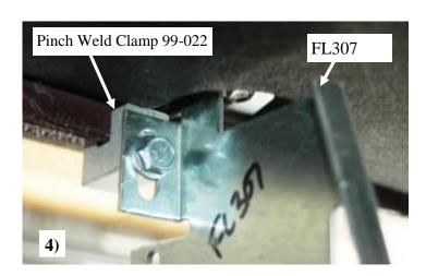
Align the rear slot on the FL307 with the tapped hole in the 99-022 pinch weld clamp mounted onto the vehicle pinch weld. Thread a 5/16 x 3/4" Flange bolt through the slot of the FL307 and into the tapped hole in pinch weld clamp.
