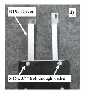
First drill through the rubber in each of the top slots of the mud flap with 5/16" drill bit. Then attach the BT97 and BT98 bracket to the rubber mud flap with two 5/16" x 3/4" flange bolts through washers and install flange nuts to rear side of the bracket.
