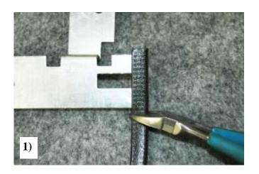
Slide the trim-lok onto bracket as shown in photo Leave approximately 1/8" extra on both the top and bottom of bracket. Cut with diagonal pliers making sure that <u>no metal</u> in extending out of vinyl. Do this to both the BT97 and the BT98 brackets.
