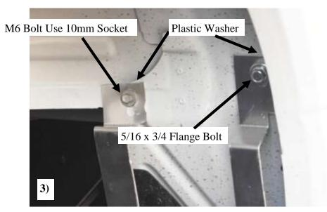
Remove the M6 bolt from just inside the rear wheel well. Place a <u>plastic washer</u> between the steel bracket and the aluminum body and install the M6 bolt that was removed into the slot on bracket, the slot is there to adjustment to level mud flap. Once the M6 bolt is snuged up to hold bracket, slide a 5/16" x 3/4" flange bolt through the other slot in bracket making sure that a <u>plastic washer</u> is in between the steel bracket and the aluminum body.
