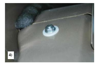
With the 5/16" x 3/4" flange bolt through the bracket and plastic washer, slide through the rear wheel well slot. On the back side of slot place a <u>plastic washer</u> onto the threads protruding through the wheel well and put a 5/16" flange nut onto the threads.
