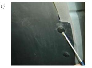
Pull inner plastic wheel well cover back and install clip nut into top hole where push pin was.
