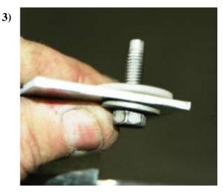
Remove the M6 bolt from just inside the splash shield that the push pin was removed in step 1. Place a <u>plastic washer</u> between the steel bracket and the aluminum body and install the M6 bolt that was removed into the slot on bracket, the slot is there to adjustment to level mud flap.
