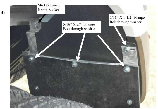
First drill through the rubber in each of the top slots of the mud flap with 5/16" drill bit. Then attach the bracket to the rubber mud flap with three 5/16" x 3/4" flange bolts through washers and install flange nuts to rear side of the bracket.
