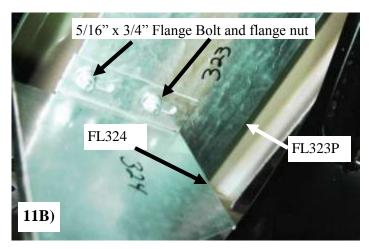
Put the FL324 bracket top slots over the two bolts coming down out of the FL323P, and secure with two 5/16" flange nuts shown in photo **11B**, Hand tighten for adjustment when boards are mounted.
