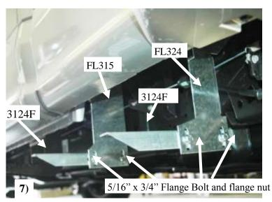
Mount the 3124F angles to the FL315 and to the FL324 lower slots with 5/16" x 3/4" flange bolts and flange nuts through each slot as shown in photo 7
