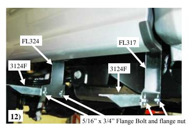
Mount the 3124F angles to the FL317 and to the FL324 lower slots with 5/16" x 3/4" Flange bolts and flange nuts through each slot as shown in photo **12**
