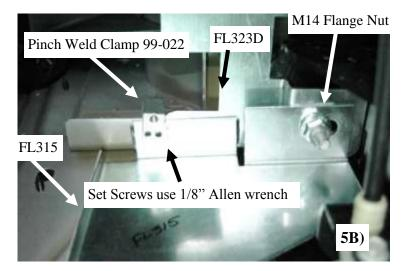
Slide the FL315 bracket up onto the M14 threads on the front bed cross brace. Thread the M14 flange nut onto the threads tighten completely, making sure the FL315 is slid all the way back in top slot use 21mm deep socket or 13/16" if a metric socket is not available.
