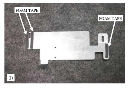
Place a strips of foam tape on the top of the both the FL323D and FL323P bracket as shown in photo, this will insulate the steel bracket from the aluminum body to avoid corrosion.
