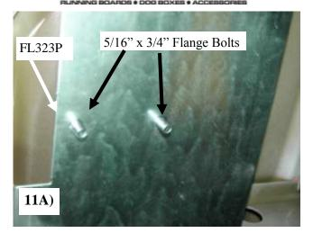
Place two 5/16" x 3/4" flange bolts down through the holes in the FL323P from the top, so the threads point downward shown in photo **11A**
