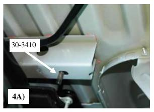
Slide the 30-3410 stud plate into the second bed cross brace so that the threads drop down through the slot in the cross brace as shown in photo 4A
