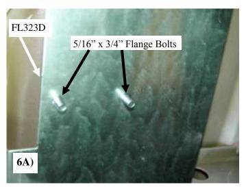
Place two 5/16" x 3/4" flange bolts down through the holes in the FL323D from the top, so the threads point downward shown in photo **6A**
