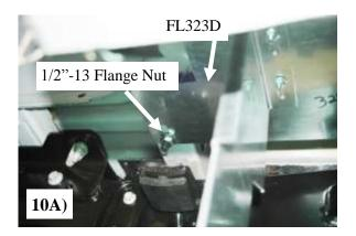
Slide the FL323P up over the threads of the 30-3410 stud plate and place a 1/2-13 flange nut onto the threads to secure. Photo **10A**
