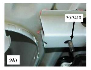
Slide the 30-3410 stud plate into the second bed cross brace so that the threads drop down through the slot in the cross brace as shown in photo **9A**
