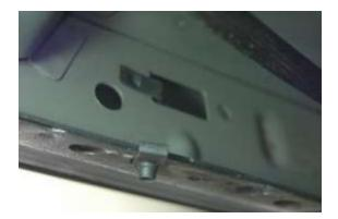
Pull the tape that covers large hole in rear of rocker panel. Slide a spring clip into hole until it snaps into the other hole.
