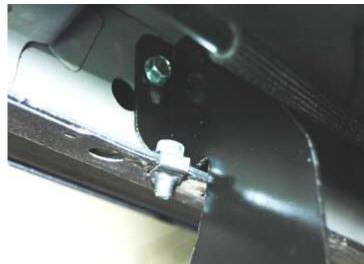
Attach brackets to vehicle by inserting a 5/16" x 3/4" bolt into the spring clip and 5/16" x 3/4" bolt and nut through the pinch weld hole.
