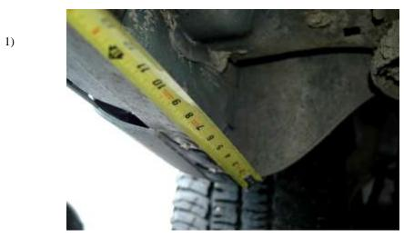
Measure from front wheel well back Std Cab—16" & 48" Super Cab—17", 33 1/2", 64" Super Crew Cab—17", 47", 70"
