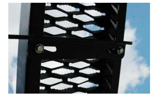
Place the board on the brackets and align up on the vehicle. Attach to the brackets using #14 X 3/4" long self drilling screws.
