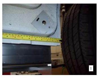
Measuring from the front wheel well back, Fig 1 mark the following locations on the pinch weld. There will be factory holes in line with these marks that will be used to mount the running board brackets
